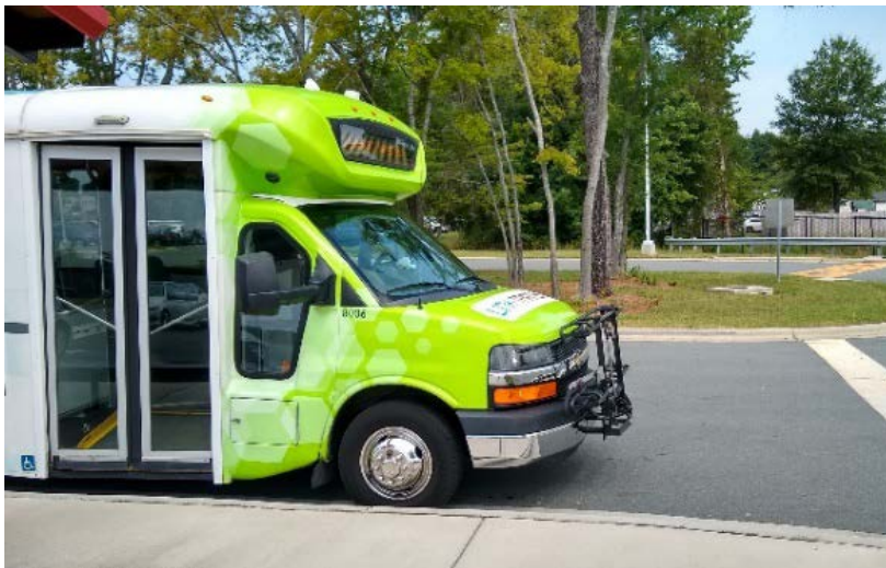
Figure 29 Link Transit Bus with Bicycle Rack on the Front
