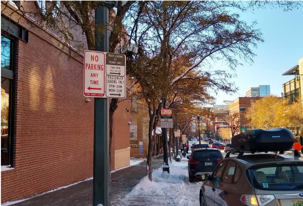
Figure 46 Dual Use Zone Dividing Time between Commercial Loading and Passenger Pick-up/Drop-off
